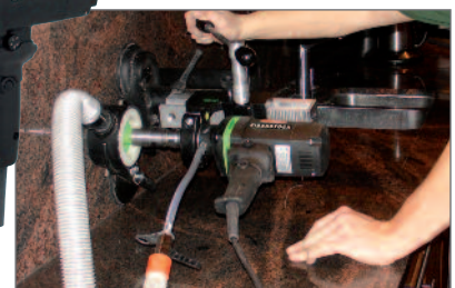
END 712 P Mini Diamond Drill for tile, natural stone and concrete Drill holes 5/32" to 3/4" 0-8000 RPM
